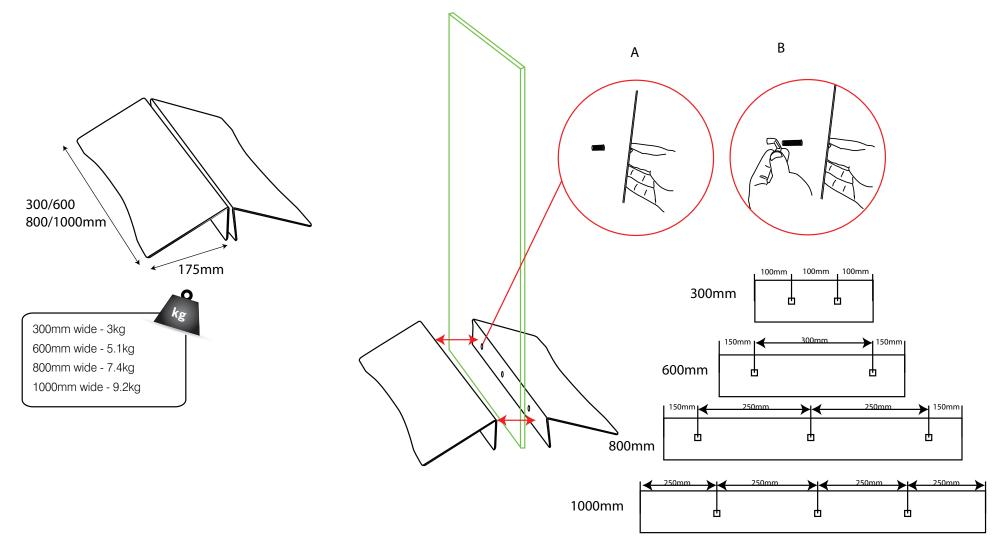
Hole height from the bottom of the unit is 42.50mm 8mm Bolt Supplied
